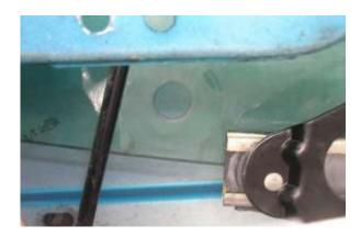
OK, now put on that new window stop guide. (The new guide should fit perfectly so that you can attach it to the window while allowing it to slide along that black vertical bar you see in the picture)
