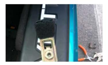
Now unbolt and remove the old L-bracket, and put the new one on. Keep a mental note of how the old bracket is attached. The Velcro on the new bracket should be facing away from you, and should be 'high' on the door. Almost think of the bracket like a Tazer gun; hold the 'bare' metal part in your hand, with the Velcro end acting as the 'barrel' of the tazer gun pointed at someone, and ready to give 'em a light little jolt.
