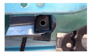
Now, just put the retainer nut on the backside of the new window guide, and bolt it into place (Remember, you'll need to use the retainer nut tool or a tool like vice grips to secure that retainer nut again so it doesn't move, etc). Do not overtighten! If you overtighten the bolt and nut, you risk breaking the window!
