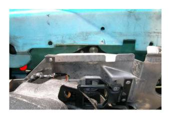
Once you have removed the sheet metal from inside the door, roll your window down about ½ way. When you do this, you should see the location of the Window Stop Guide (highlighted in red.)
